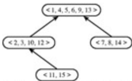
(e) The result from each of these four supervertices choosing its minimum-labeled neighbor
