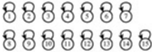
(b) The initial forest consisting of a distinct tree representing every vertex in V
