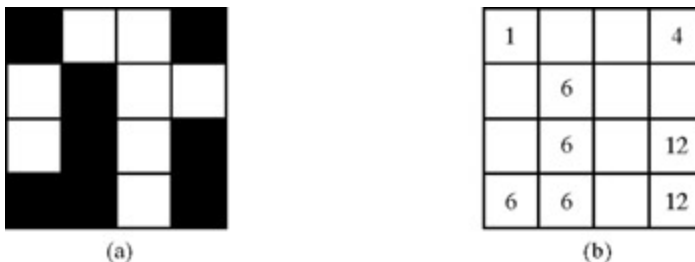
Figure 11.1: (a) A digitized 4 \times 4 picture. The interpretation is that it is a black image on a white background. (b) The same 4 \times 4 picture with its maximally connected components labeled under 4-adjacency definition of connectedness. Each component
