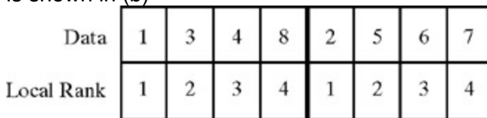
Figure 9.3: A snapshot of MergeSort on a linear array of size 8, using the data from Figure 9.2 . The snapshot shows the data and local ranks that are determined after the independent sorts on both the Left and Right subarrays
