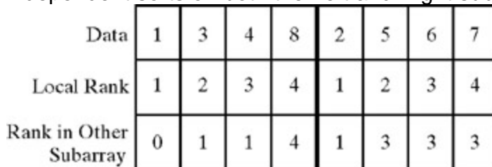
Figure 9.4: A snapshot of MergeSort on a linear array of size 8 after the independent sorts on both the left and right subarrays. The data, local ranks, and ranks with respect to the opposite subarray are all given. The data is from Figure 9.2
