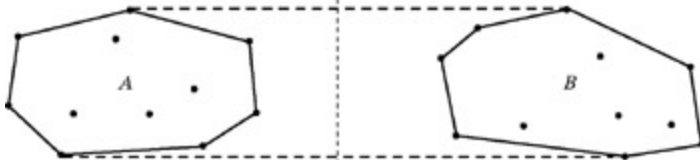
Figure 10.9: The stitch step. To construct \text{hull}(S) from \text{hull}(A) and \text{hull}(B) , the upper common tangent line and lower common tangent line between \text{hull}(A) and \text{hull}(B) are determined
